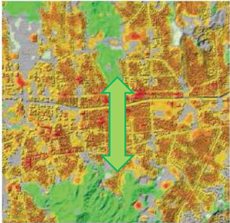
Fig.4.5 Air temperature of the study site and surrounding area the air temperature of surrounding Seunsangga buildings is particularly higher
